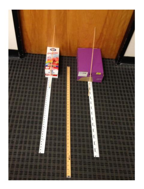
Students had "ladders" (sticks) and boxes. They measured how high their "ladders" reached the wall, and how far from the wall the ladder touched the floor, to see how well the theoretically derived predictions matched the actual measurements.
