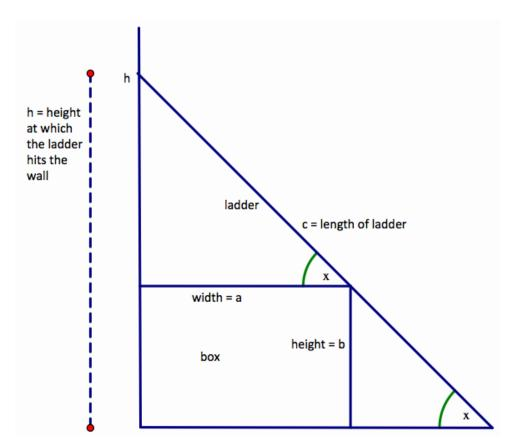
The general solution for a box whose sides have lengths a and b, and whose ladder has length c, can be obtained by solving for x the equation:
